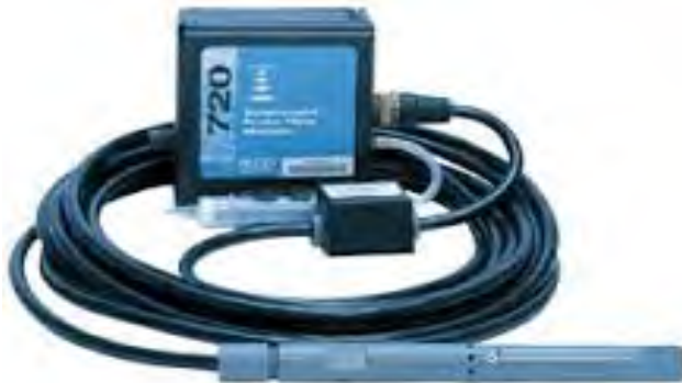
Photo 5. ISCO 6712 portable automated water sampler that integrates runoff water quality sampling with a with stage (water height at calibrated point within the flume) determination accomplished with an ISCO 720 flow module that utilizes a submerged pressure transducer within the trapezoidal flume to measure runoff discharge. The unit is powered by two 12-volt deep marine batteries in parallel and recharged by a solar panel.
