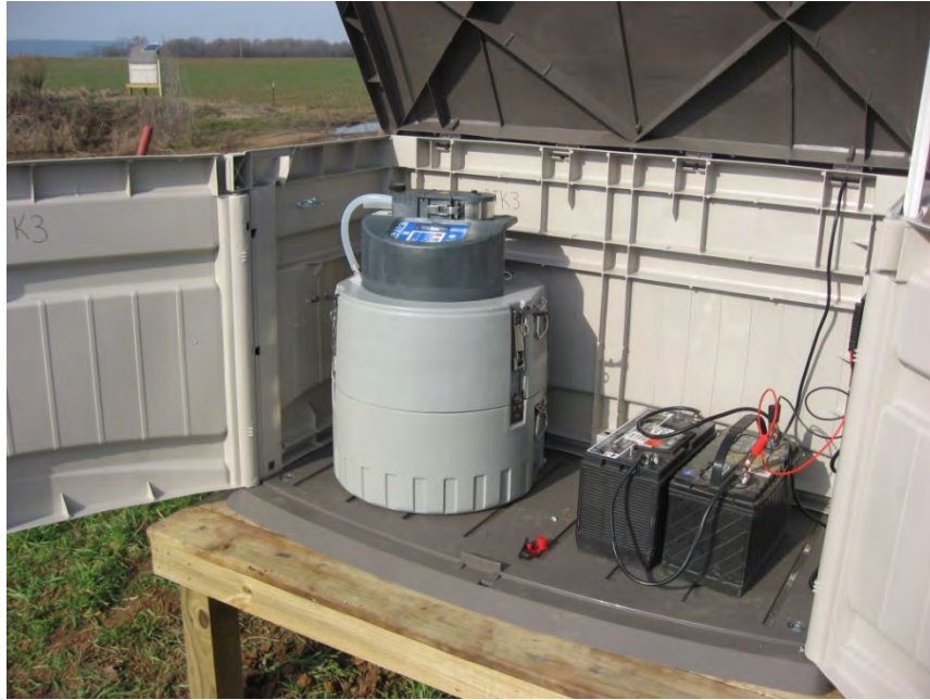
Sampling equipment at each monitored site. ISCO 6712 auto samplers will be used at all sites coupled with an ISCO submersible pressure transducer.
