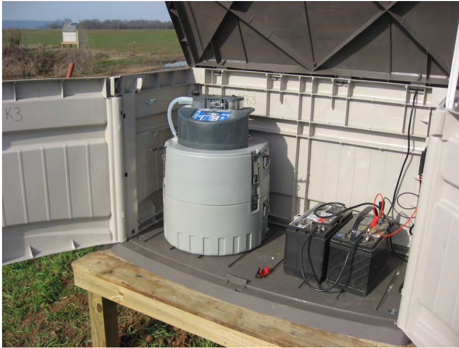
Photo 5. ISCO 6712 portable automated water sampler that integrates runoff water quality sampling with a with stage (water height at calibrated point within the flume) determination accomplished with an ISCO 720 flow module that utilizes a submerged pressure transducer within the trapezoidal flume to measure runoff discharge. The unit is powered by two 12-volt deep marine batteries in parallel and recharged by a solar panel.
