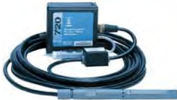
Photo 6. The ISCO 720 flow module equipped with a submerged probe that contains a pressure transducer that determines stage height above a set point.
