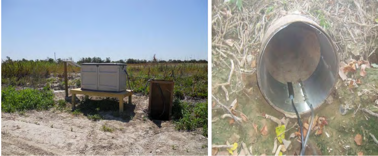
Photo 6. Prototypical monitoring station set up for the new CVW3 and CVW4 stations that will be established on the Mike Wood farm in 2014. The ISCO sampler will be housed in a storage shed attached to a wooden platform (left) and the area velocity flow meter and sampling tube and strainer will be installed into the drainage pipe and secured using a friction-fit scissor ring (left).
