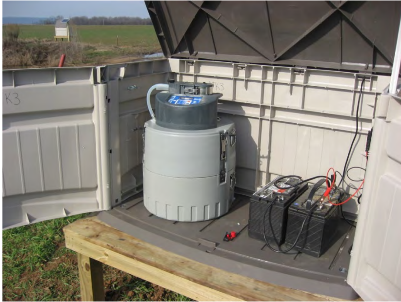
Photo 7. ISCO 6712 portable automated water sampler that integrates runoff water quality sampling with a an ISCO 750 flow module that utilizes an area velocity flow meter equipped with sonar to determine both stage height and flow velocity within an open-channel pipe. The unit is powered by two 12-volt deep marine batteries in parallel and recharged by a solar panel.
