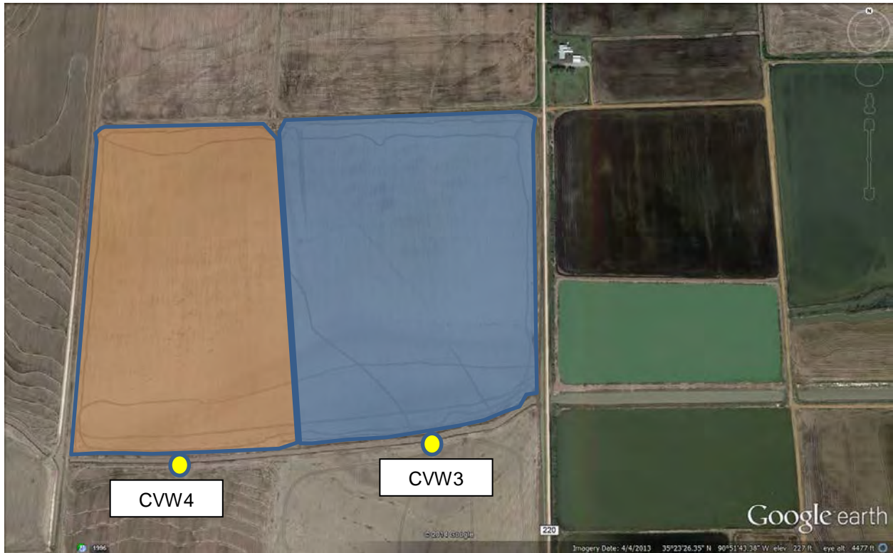
Photo 3. Close-up on new monitoring sites on the Mike Wood farm. The field currently has two outlets and will be subsequently divided into two distinct management units so that a control and selected irrigation water management practices can be compared for the effect on nutrient and sediment losses in runoff as well as water use and loss.
